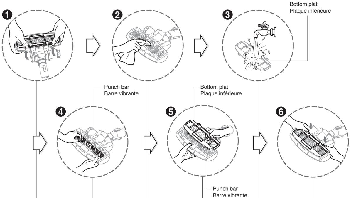
**1** Press the button on the rear side of the vacuum nozzle to separate the bottom plate.
