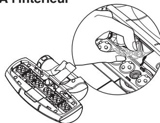
You can remove dust by hand, if you can't remove dust which is inside of nozzle by crevice tool.
