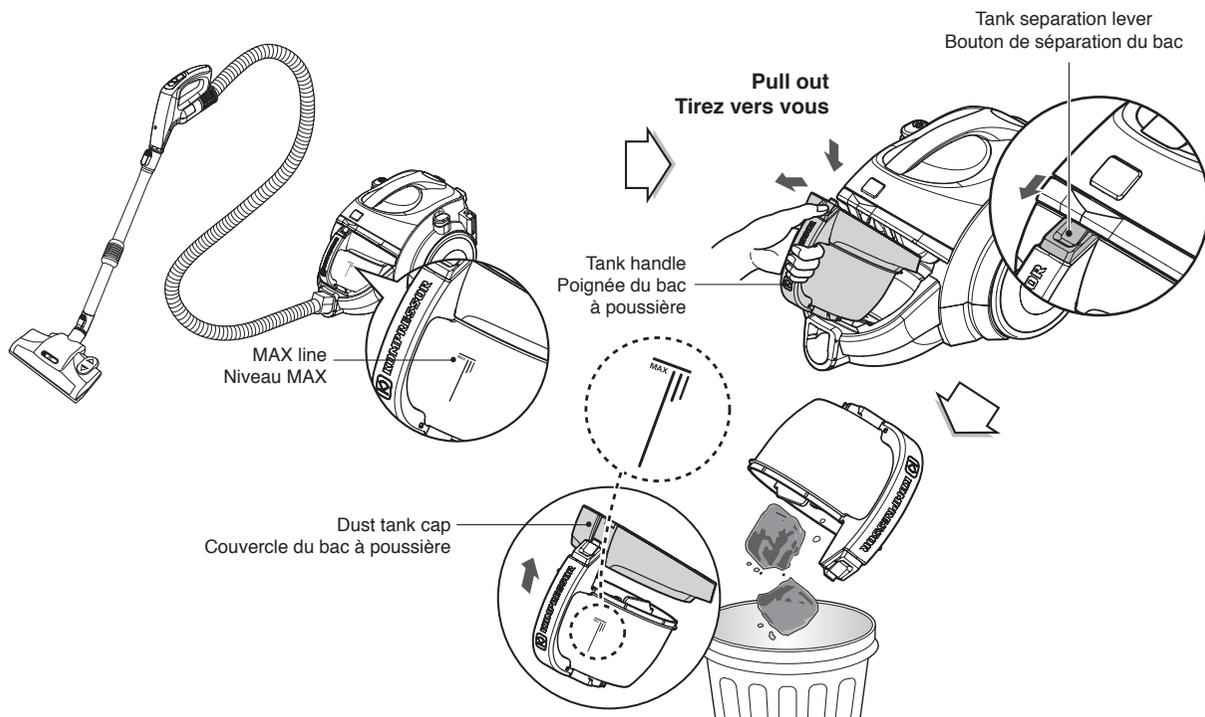
The dust tank needs emptying when the dust tank level reaches the MAX line.
