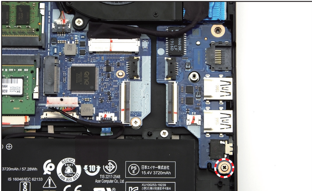
Figure 1-18. Retirer la vis
