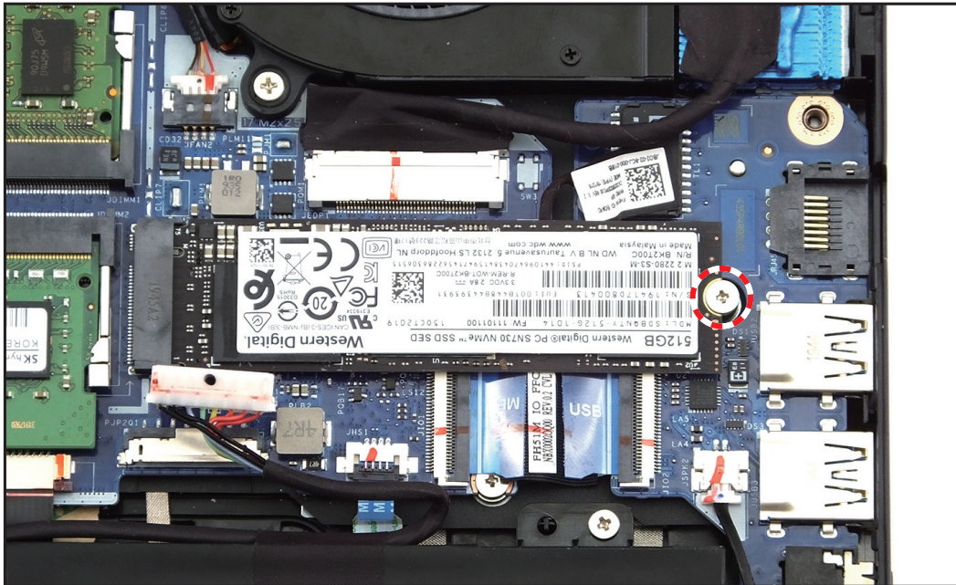
Figure 1-15. Retirer la vis
