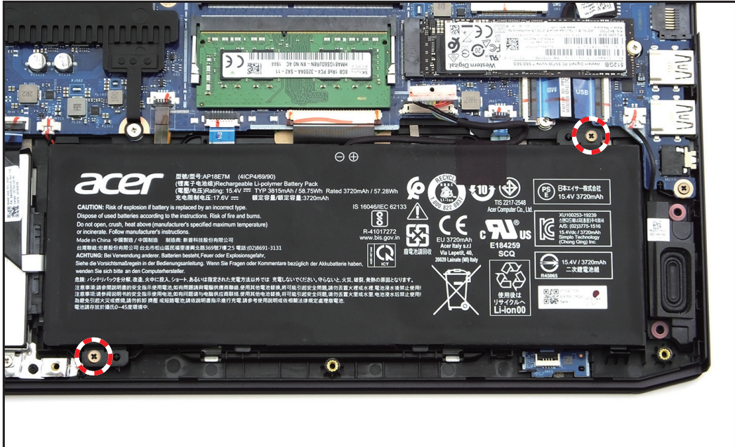
Figure 1-6. Retirer les vis
