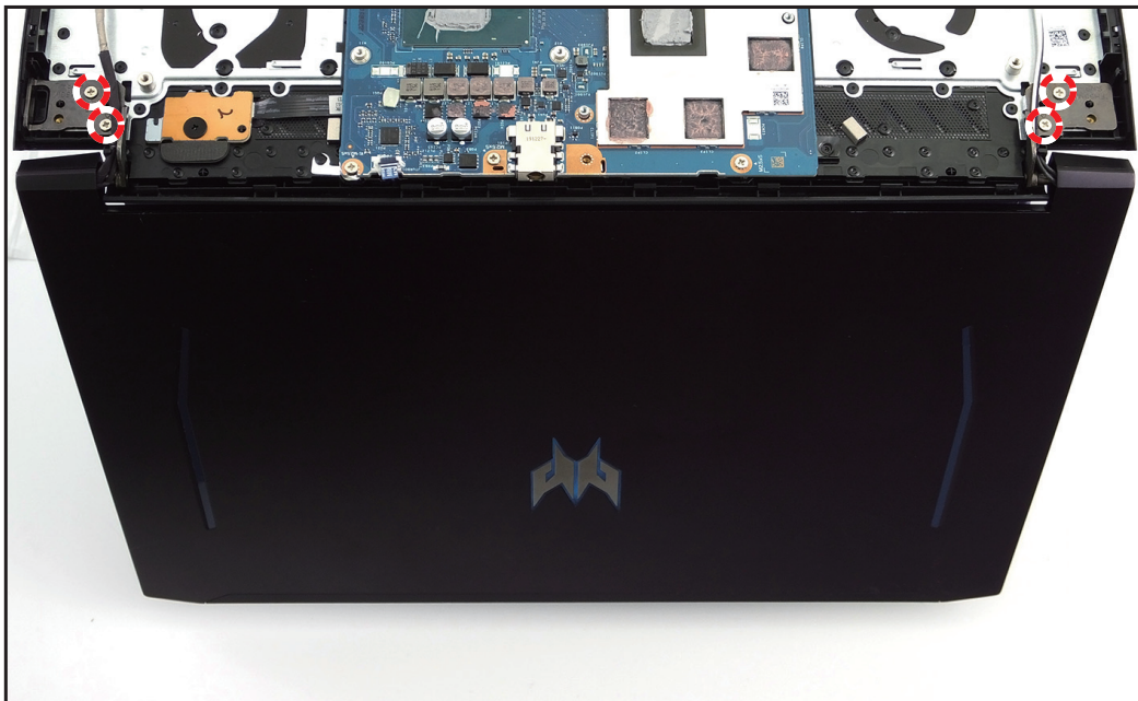
Figure 1-20. Retirer les vis
