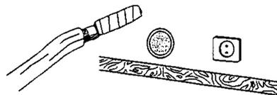
GB Protect quick coupling (on flexible tube and outdoor unit) with plastic plugs supplied as accessories. To insert the tubing into the hole in the wall easily and without damage, join the pipe ends and wrap them with adhesive tape.
